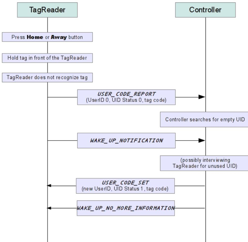
**Note:** the Tag code in above diagram is not the actual RFID TAG code but transformed to a ASCII binary digit code. You should use this binary code also in the USER\_CODE\_SET command to store it in the Tag Reader 500
