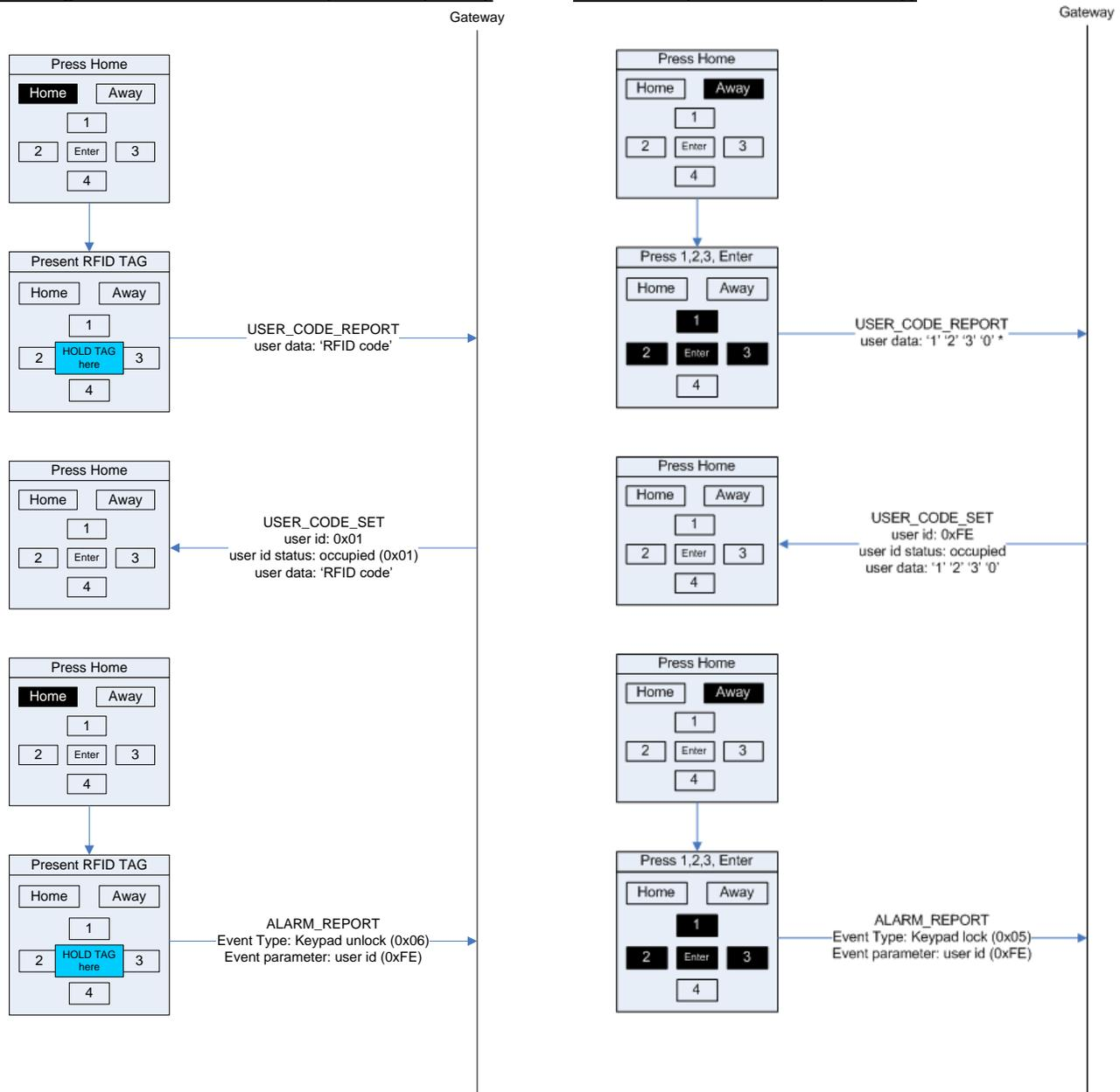
\* If a USER code is smaller than 4 digits , the value is supplemented with ASCII 0 (value 0x30) to reach a 4 digits code. Any USER code with size 4 or more will be reported with the length of the USER\_CODE.
