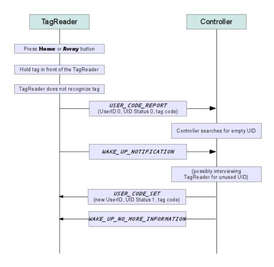
**Note:** the Tag code in above diagram is not the actual RFID TAG code but transformed to a ASCII binary digit code. You should use this binary code also in the USER\_CODE\_SET command to store it in the Tag Reader 500
